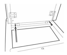
4. Attach the guard rail on the inverter stand to the printer using 2 screws.
